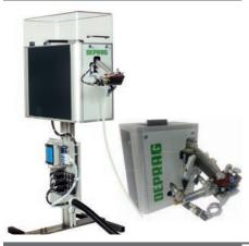
Sword feeders or segment feeders are used when the requirement calls for gentle, almost noiseless feeding of sensitive fasteners. Our sword feeder systems can process screw sizes from M2 to M6. They are ideal for screws up to 25 mm in length. Sword (segment) feeders are also well-suited for the processing of balls and pins.
