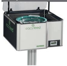
Stationary feed systems for the processing of small components of all kinds, such as screws, pins, bolts, rivets, nuts, washers and o-rings. Vibratory feeders feature a high output rate in comparison to other feed systems.
