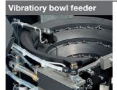
DEPRAG feeders with a vibratory drive are particularly suitable for screws from < M1 to M8.
