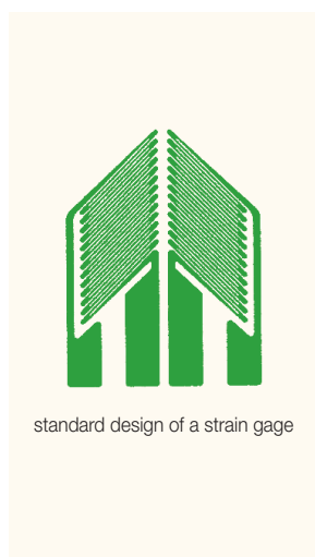
Function principle of the strain gage transducers
