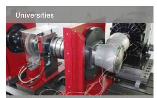
Sophisticated drive technology requires innovative sensor technology. In the field of torque and lateral force measurements, WITTENSTEIN sensors are unique. Easy integration and simultaneous recording of 4 measurement variables (M; Fx; Fy; T) are top-notch product properties. Connectivity is available via USB, analog interface and field bus – thus there are no limits to creativity.
