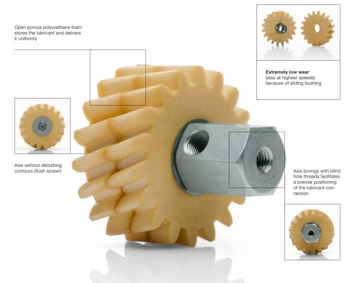
Lubricating pinions and axles perfectly harmonized with the pinion steering rack systems:
