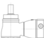
Mounting position V3/B5 (output shaft upwards, motor shaft horizontal)
